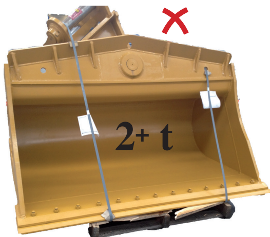
Heavy individual item with sharp edges
